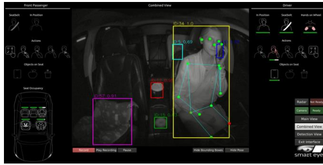
Fig 6: This figure demonstrates the intelligent driver-monitoring interface used for facial landmark tracking, seating-position analysis, and behavioural observation. The system continuously evaluates driver posture, head movement, and in-cabin activity to improve fatigue-awareness accuracy.
